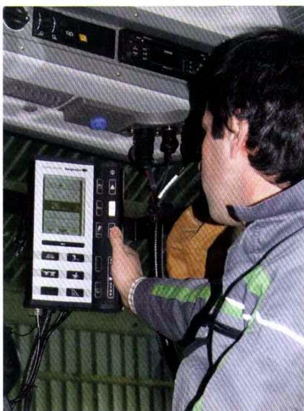
The KRM Zurf controller is used to plan, control and record all applications
