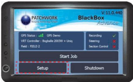
**Step 1** - On the home screen press **Setup** > **Advanced** > **Boom Section Control**.
