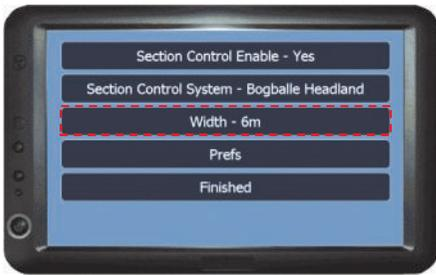
**Step 4** - Set the required working width.
