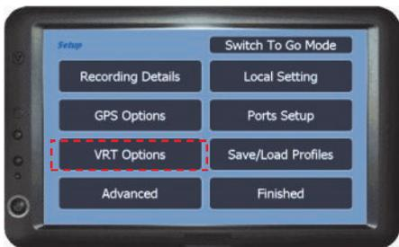
**Step 8** - Press **VRT Options > VRT Test**, then power up the spreader controller and put the spreader into full working mode (It is advised that the test is done with no product in the spreader).
