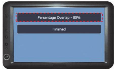
**Step 5** - Press **Prefs > Percentage Overlap**, set the overlap to '50%' and when complete press **Finished x3**.
