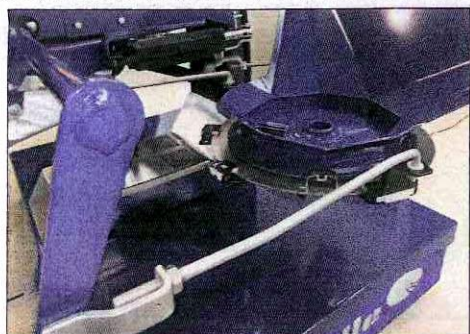
To make Section Control Dynamic work it requires dual shutters on both discs to alter drop on point and application rate.
