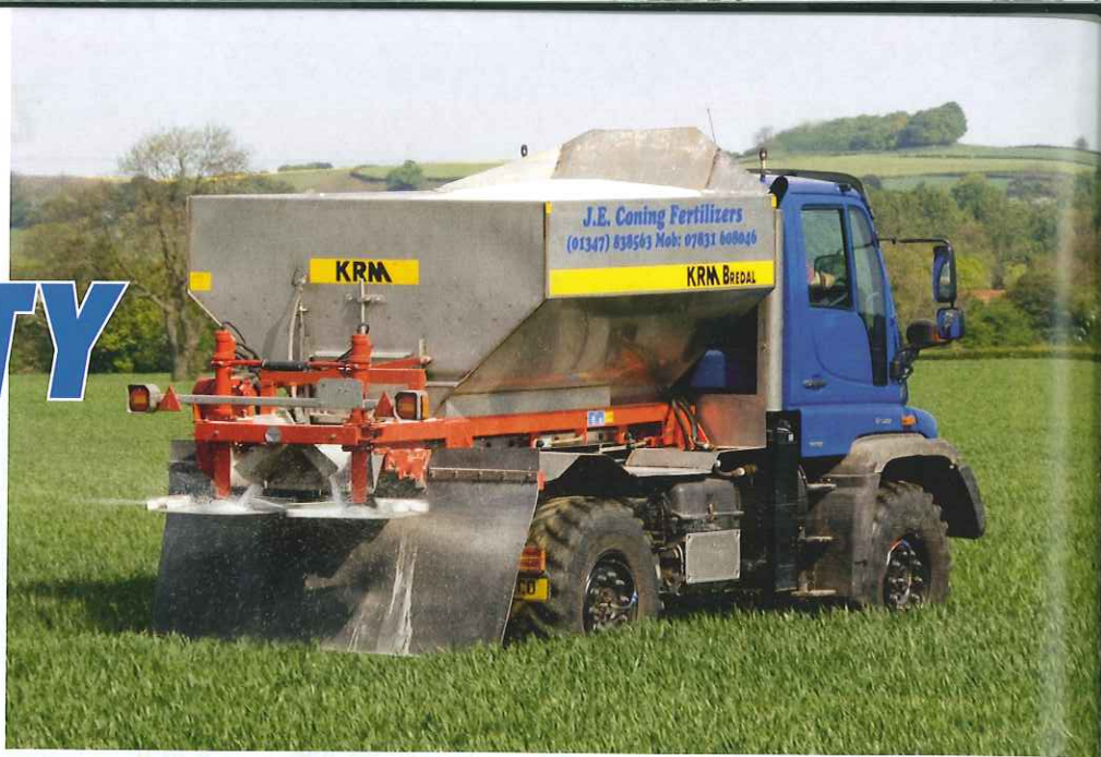
Coning Fertilizer Ltd's modifications to its new KRM Bredal twin disc spreader have increased its capacity, while lowering the centre of gravity to increase safety when working on steep land.
