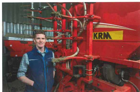
TOP Mr Canvin's 6m model boasts a 2,000-litre pressurised hopper yes is compact enough to travel along narrow lanes
